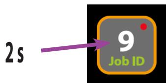
Press and hold option button for 2s. Top display will show abbreviation of selected option. In bottom display user can see current value.
